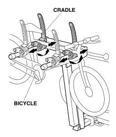
2. Install the two anti-sway cage assemblies to the bicycle arms as shown.
